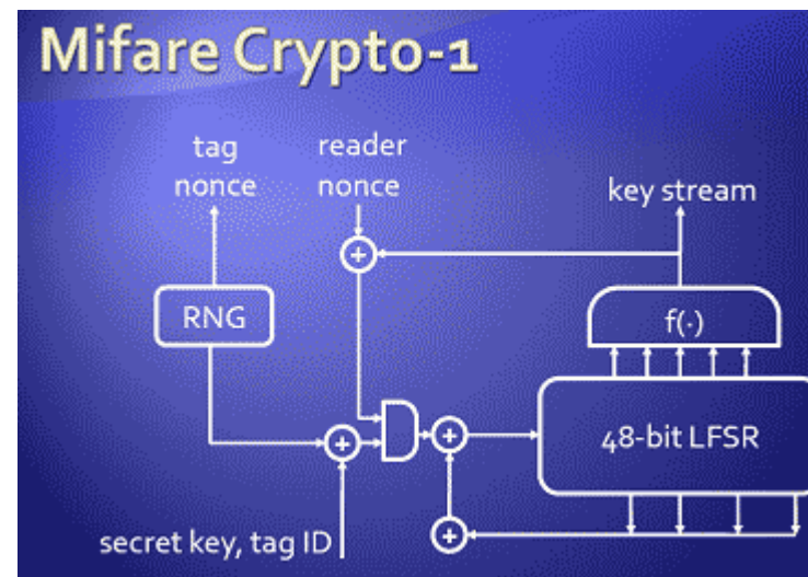
Mifare Crypto-1 - Logical view of secret algorithm – (Reverse engineering – Electronic Low level analysis) – Source: CCC 2007 – Mifare Security
